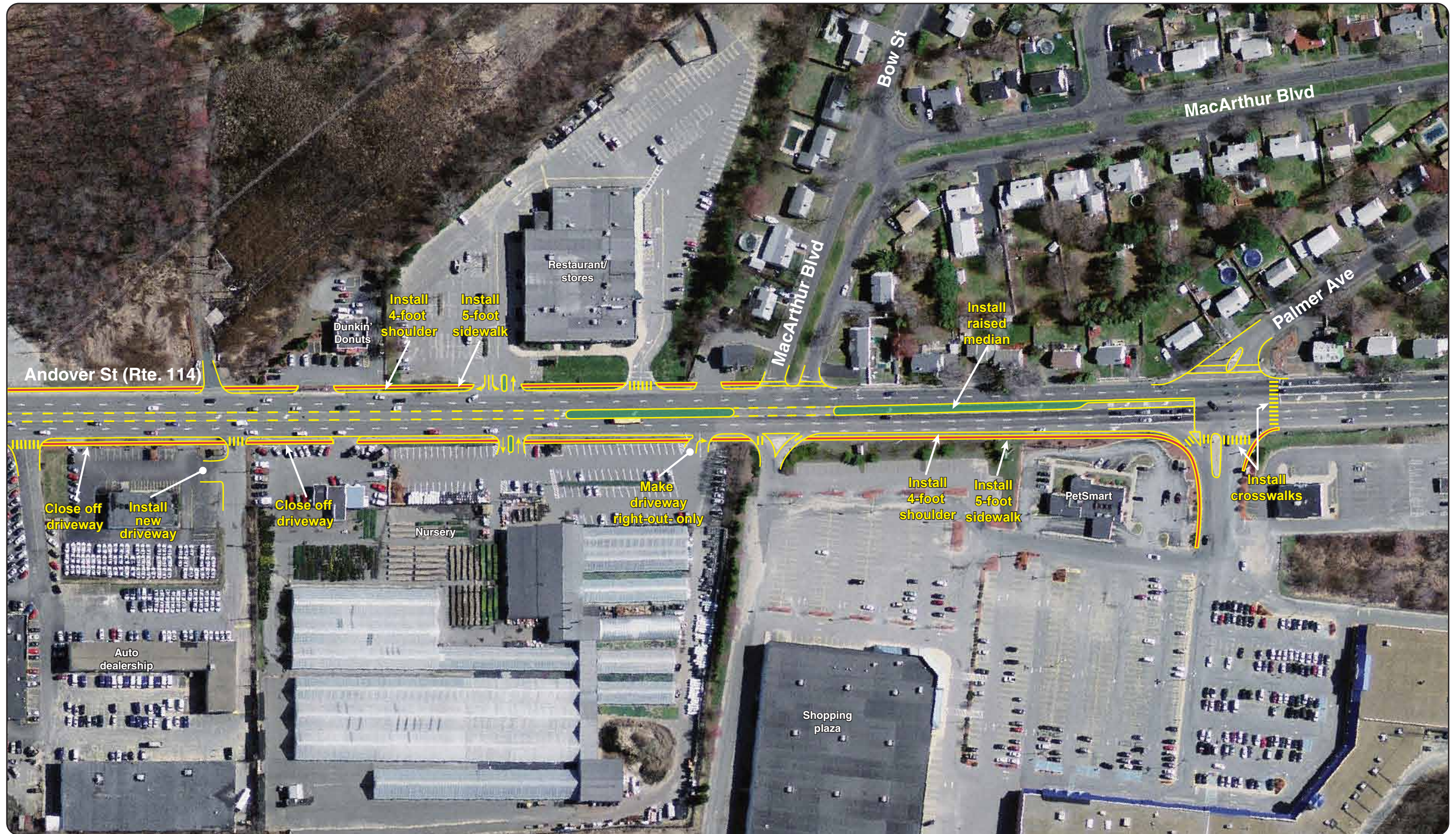
FIGURE 14 Proposed Long-Term Improvements – Alternative 2 Conceptual Plan (Eastern Section)
