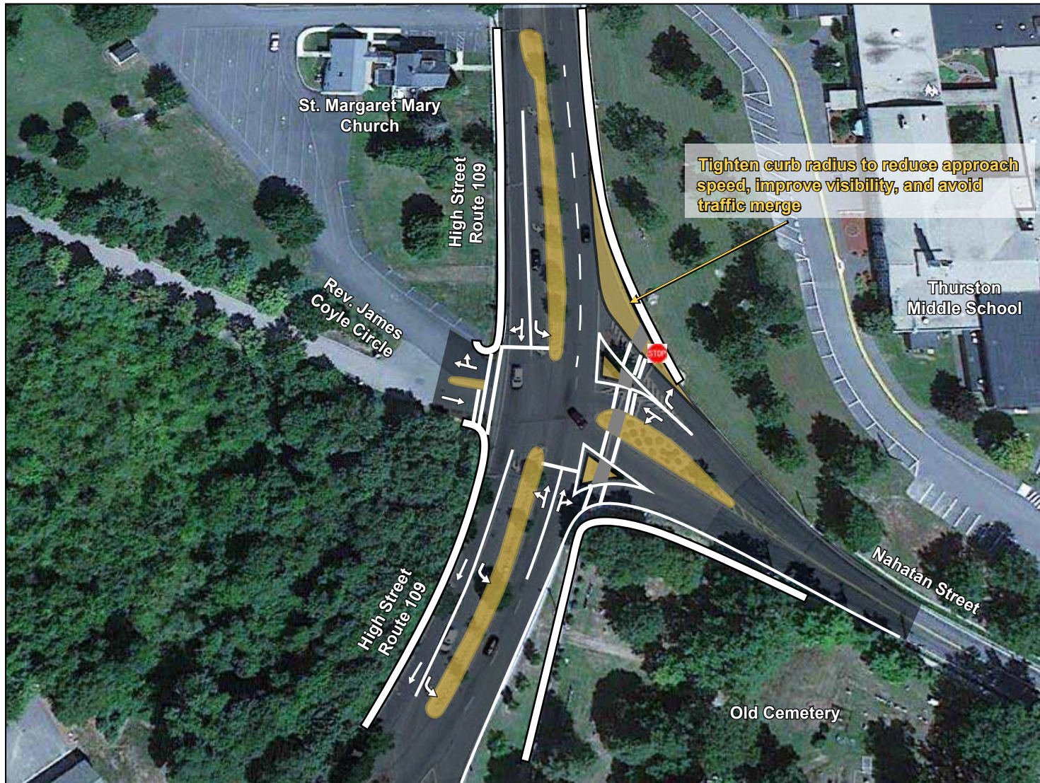
FIGURE 7 Medium-Term Improvement: Alternative 4 Tighten Curb Radius for Nahatan Street Right-Turn Lane
