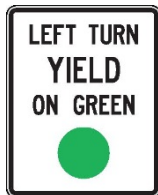
R10-12, Traffic signal sign
